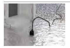
COMPAC pumps are submersible pumps for clear water, equipped with an asynchronous single-phase motor and with a stainless steel motor shaft (anti-corrosion). The integrated check valve placed on the discharge prevents water from flowing back to the pump.
