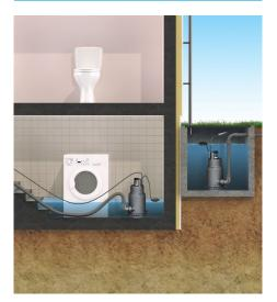
Submersible pump for clear water drainage, equipped with float switch for automatic operation and with ergonomic handle for a secure grip and an easy portability. Thanks to cooling jacket the pump can work in both immerged and submerged conditions. The flat suction device allows to drain water down to 2mm
