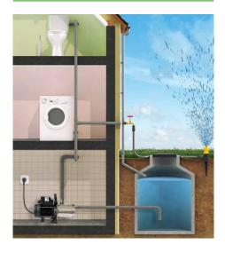
EVOTRONIC 350 is a system composed of a multistage self-priming pump, with stainless steel pump body and an electronic frequency changer (inverter) that, according to the effective water demand, allows the pressure to be maintained constant in the system, reducing or increasing the electric pump motor rotation speed.
